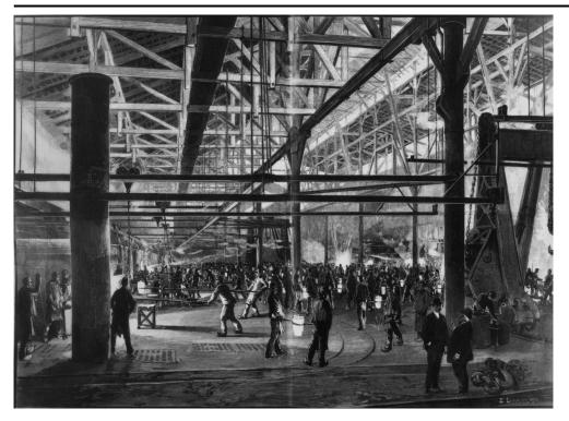
Source: "Im Schmelzbau"—Tiegelstahlguss in der Gussstahlfabrik Krupp in Essen ["Im Schmelzbau"—Crucible Steel Casting at the Krupp Cast Steel Factory in Essen]. Woodcut based on a drawing by Emil Limmer (1890).
